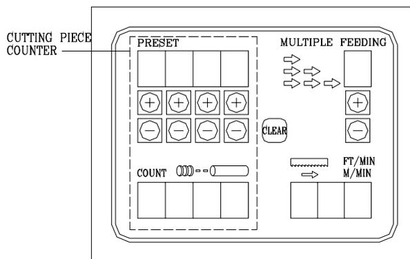
**Cutting Piece Counter** – This counter is used to preset the number of cuts required on the automatic operation. When the counter reaches the preset number, the machine stops automatically . To activate the counter, preset the counter switch with number at least “1”.
