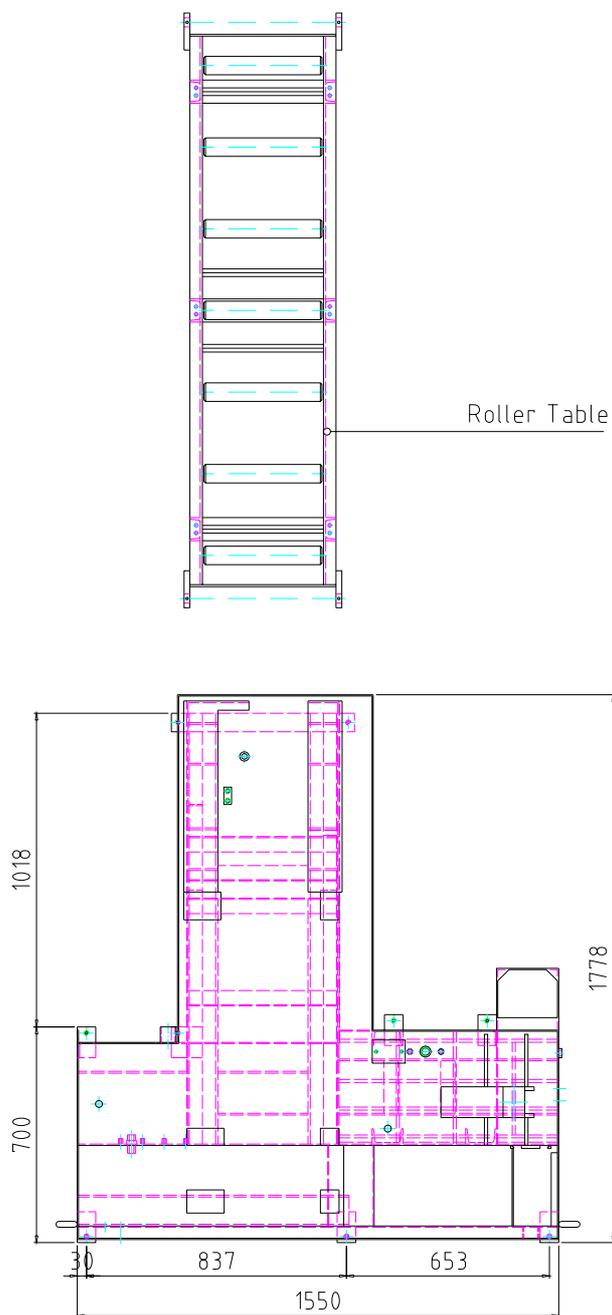
The position of anchor bolts and floor dimensions are shown in fig 4:
